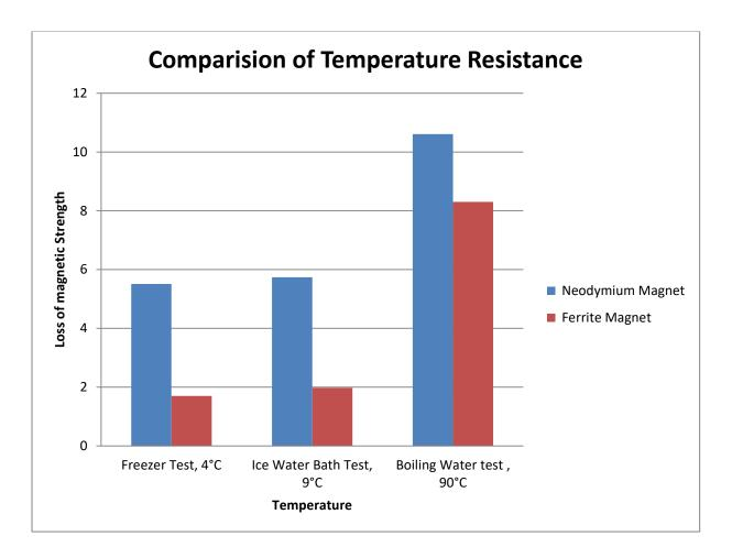
The above graph shows that even though the magnetic strength is higher in neodymium magnets, it lost more magnetic strength when treated under extreme temperatures compared to ferrite magnet.
